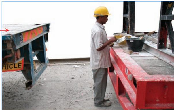
Pre-loaded trailer which lurched backwards crushing the worker standing behind
