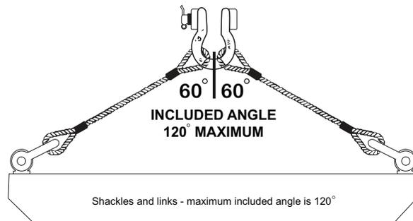
When lifting is done with fixed length multi-legged slings, any two legs of the slings must be capable of supporting the total load of the pre-cast component.
