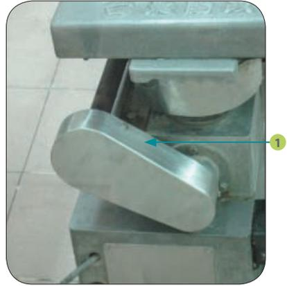
1 In-running nip of belt and pulley is fully enclosed to prevent hand and finger injuries
