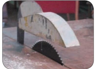
Saw guard must be adjusted as close to the timber piece as possible before cutting operation
