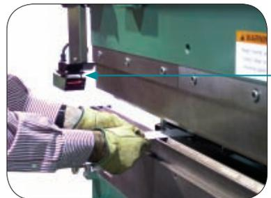
1 Press brake installed with laser sensing system that has transmitter and receiver mounted below the RAM to cut off power supply to prevent hand and finger injuries (Picture courtesy of Omron STI)
