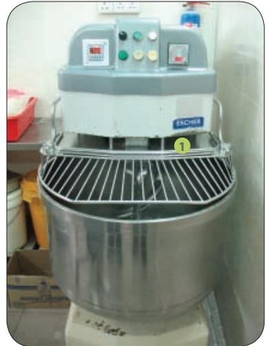
1 Flour mixer installed with interlocked guard
