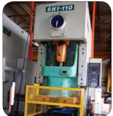
Light curtain not properly positioned to prevent operator's hands and fingers from straying into danger zone of the hydraulic power press
