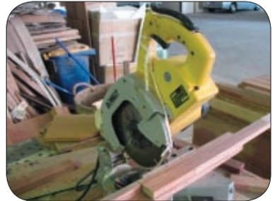
Defective guard must be repaired or replaced
